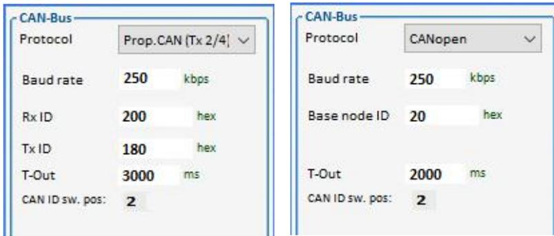
**Figure 6** The CAN group with CAN and CAN open firmware
