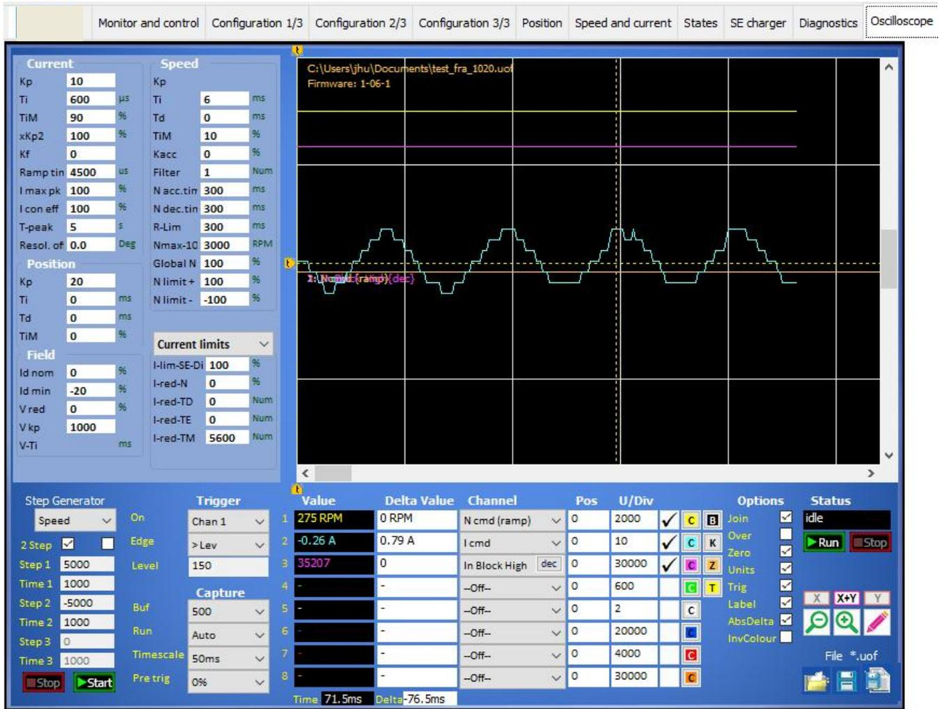
Figure 15 The built-in oscilloscope
