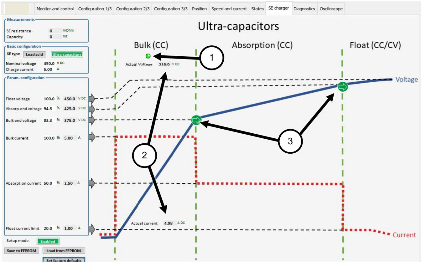
The illustration on the right shows the charging process used for the selected SE type. The LED (1) shows which state is active. When the charger is charging, the actual voltage and charge current are shown in the active state (2).
