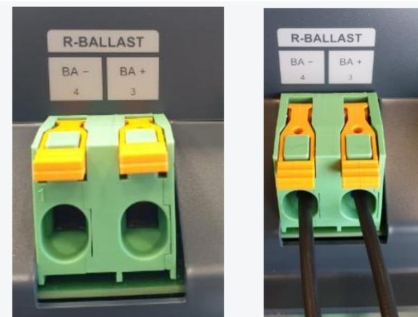
Connect the resistor's wires to the IMD X1 R-BALLAST connectors according to the wiring diagram and the instructions in section [5.2.1](#) on page [28](#).
