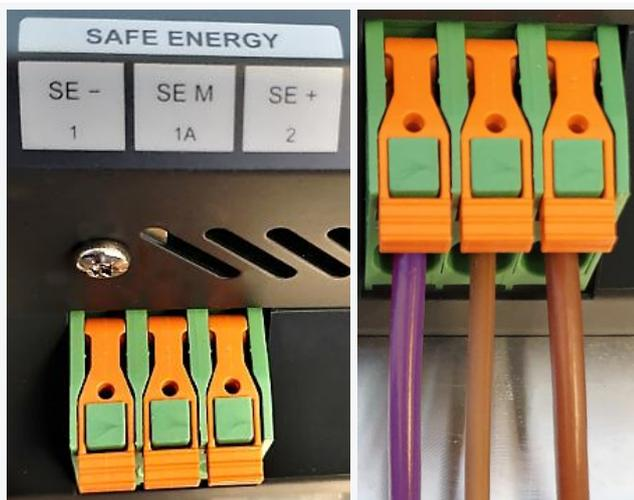
Connect the battery or Ultra Cap wires to the IMD X1 SAFE ENERGY connectors according to the wiring diagram and the instructions in section [5.2.1](#) on page [28](#).
