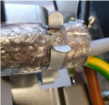
2. Fasten the cable with cable ties on both sides of the shielding clamp:
