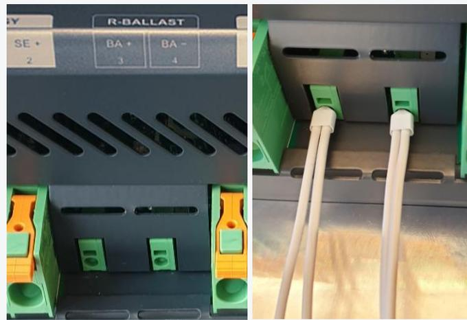
Connect the resistor's wires to the IMD X1 R-BALLAST connectors according to the wiring diagram and the instructions in section [5.2.3](#) on page [30](#).
